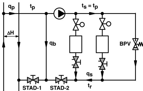
This method is only applicable if the flow measurement device is of the variable orifice type, as the STAD balancing valve.
