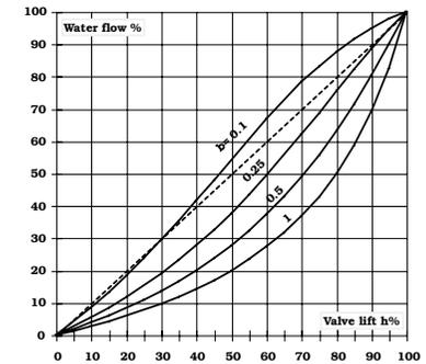
*Distortion of the "EQM" characteristic of a valve as a function of its authority.*
