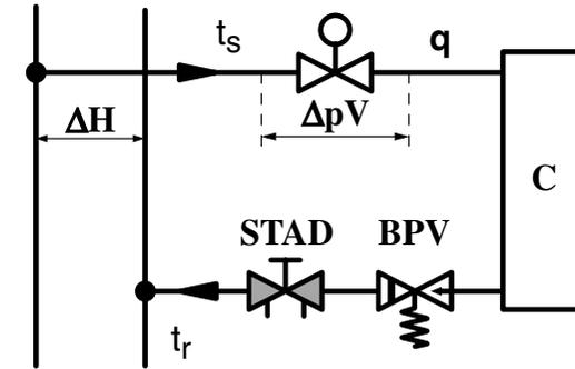
Fig. 2. A modulating relief valve reduces the differential pressure by a constant value regardless of the flow.
