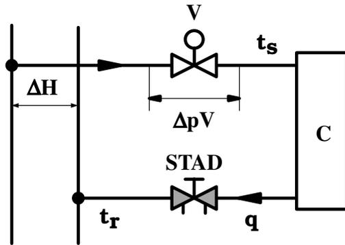
Fig. 1. Control of a variable flow terminal unit
