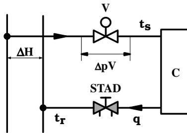
*A balancing valve limits the flow in the control valve without changing its authority  $\beta'$*
