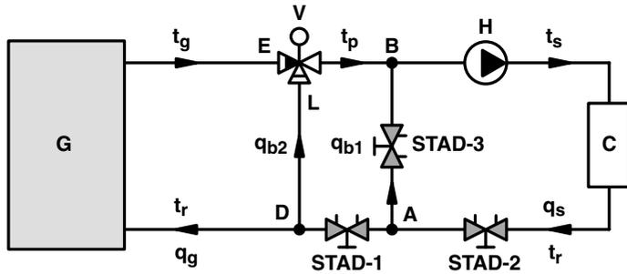
Fig. 16. Mixing circuit with intermediate bypass.
