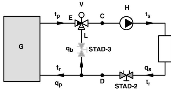
Three way valve in mixing function.
