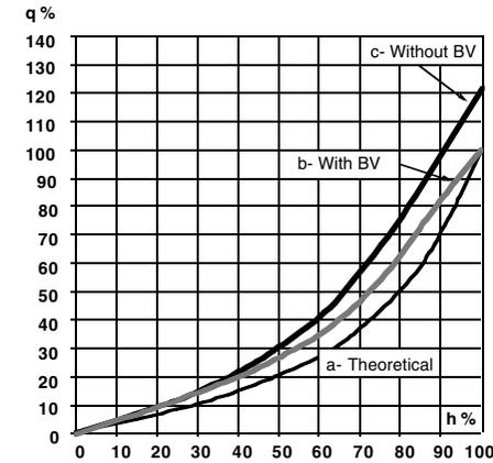
Influence on the control valve characteristic through limiting the maximum flow by a balancing valve.
