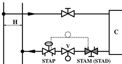
*A  $\Delta p$  controller keeps constant the differential pressure across the control valve*
