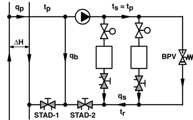
Fig. 13. Reducing or increasing the differential pressure applied across coils by means of a secondary pump.
