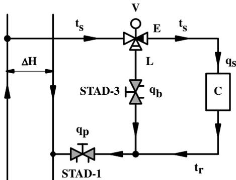
*Diverting valve mounted in a diverting circuit.*
