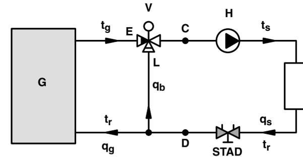
Fig. 15. Mixing circuit associated with a production unit.
