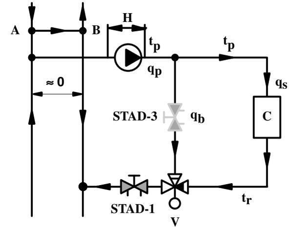
Fig. 23. Circuit in diversion on a passive distribution.
