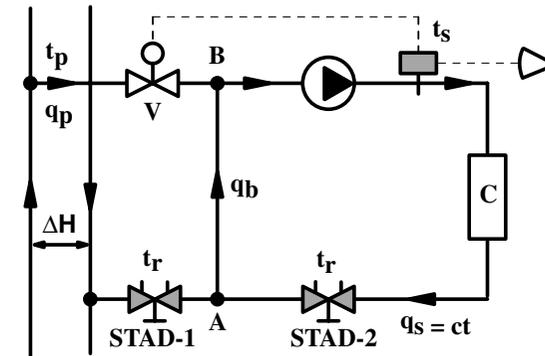
Fig. 8. Control of coil output for a coil supplied at constant flow.
