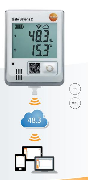
The WiFi data logger system testo Saveris 2 is the modern solution for the monitoring of storage and work rooms. The system consists of WiFi data loggers and a Cloud data store.
