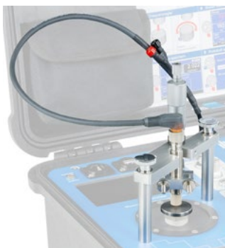
◀ CV-10 with adapter for proximity probes
