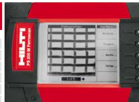
An Imagescan displayed on the monitor for on-the-spot analysis of reinforcement (location, depth, diameter).
