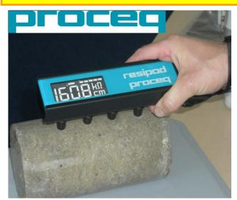
Surface resistivity measurement provides extremely useful information about the state of a concrete structure. Not only has it been proven to be directly linked to the likelihood of corrosion and the corrosion rate, recent studies have shown that there is a direct correlation between resistivity and chloride diffusion rate.
