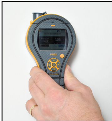
Figure 3: Taking Relative Moisture Readings
