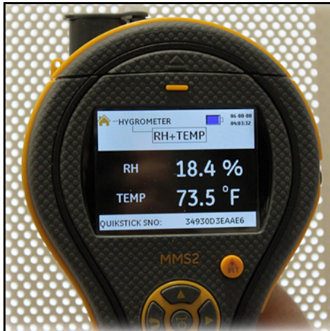
Figure 4: MMS2 as a Hygrometer
