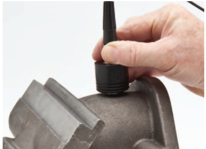
Many cast metal parts or sound-attenuating materials can be measured with the High Penetration software option.
