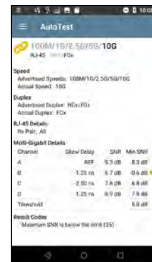
Cabling SNR measurement validates Multi-Gig links
