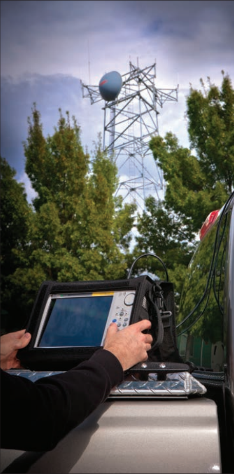
LMR Master testing from a service vehicle
