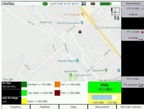
PTC ACSES Coverage Mapping RSSI, EVM, and BER on map
