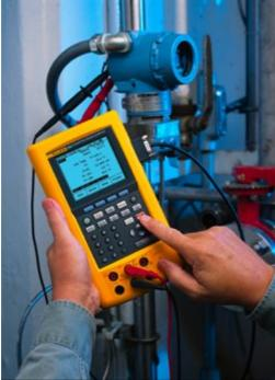
The 744 is a power multifunction documenting calibrator that lets you download procedures, lists, and instructions created with software-or upload data for printing, archiving, and analysis. The 744 also features a powerful built in HART® interface capable of performing nearly all the day-to-day tasks you now perform with a separate communicator.
